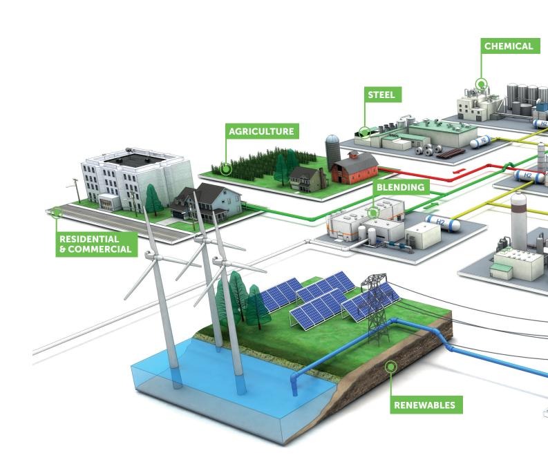
Power-to-X describes the process of converting renewable energy into hydrogen via water electrolysis. The produced green hydrogen can then be used as a fuel or feedstock in a variety of applications, many of which renewables alone have a hard time penetrating. Green hydrogen acts as the bridge between renewables (Power) and a multitude of downstream sectors (X).
